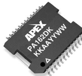
20-pin PSOP PACKAGE STYLE DK
